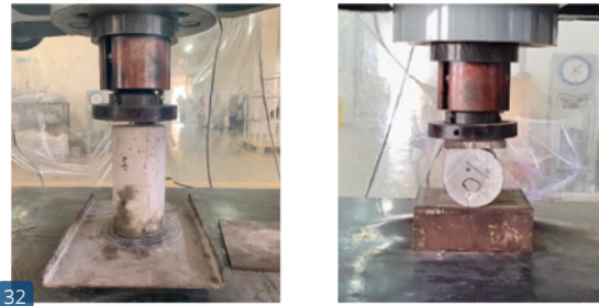
a. Compressive strength test b. Splitting tensile strength
